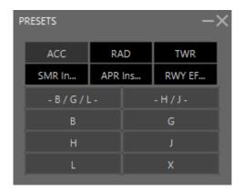
There are 6 different groups, all accessible via the black buttons. The correct preset for the ATC position is automatically loaded when signing in, however you may change it manually in this menu.
